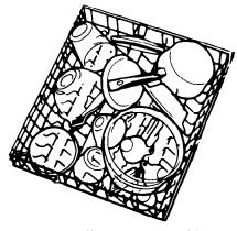
Load correctly for best washing results. Incorrect loading may cause poor washing and the need to rewash all or part of the load.
